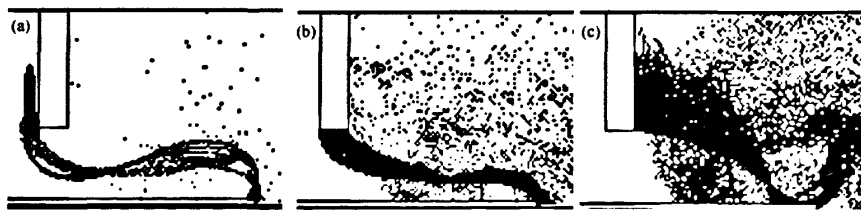
图 5 磁限制阶段阴极不同表面发射电子束的箍缩状态 (a) 后表面, (b) 中间表面, (c) 前表面 Fig.5 Pinching schemes of electrons emitted from different surfaces in ML phase. (a) Upstream, (b) Middle, (c) Downstream
